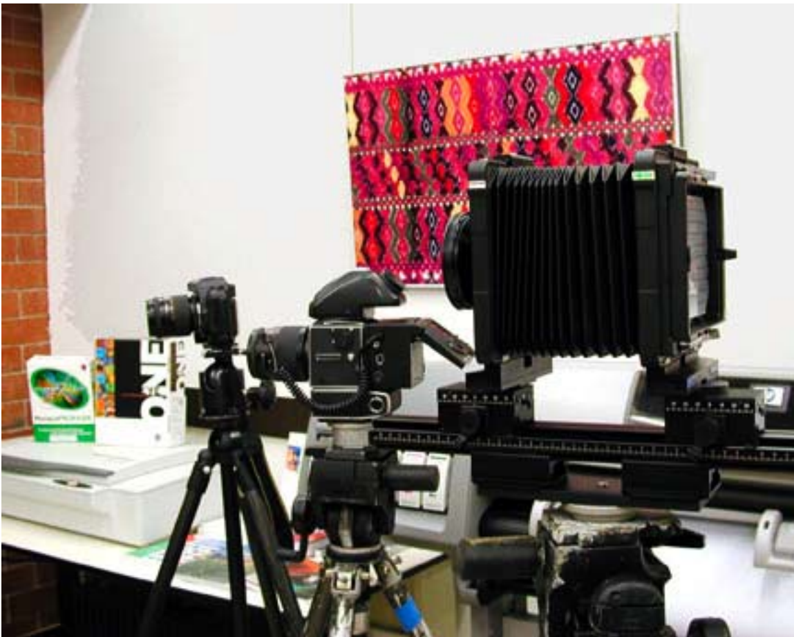
Three levels of digital cameras at FLAAR ready for testing for use in the course by Nicholas Hellmuth: 35mm SLR Nikon D-100, medium format Hasselblad with Kodak Pro BackPlus; 4x5 with BetterLight scanning back.
